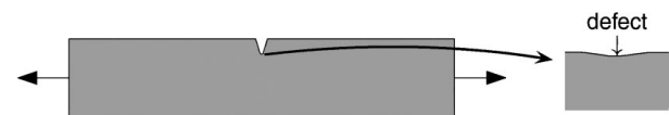
Figure 8 Plane strain model of a notched tensile test specimen with a minor defect at the blunt notch tip.
